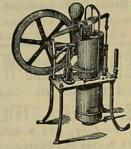
is especially intended for domestic use in lifting and forcing water from wells and cisterns, or from Oroton pipes, to tanks on upper floor of buildings in city or country. Absolutely safe. Servant-girl can operate; 18 feet gas per hour.
