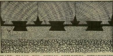
Composed of wood blocks, ce mented and keyed to concrete foundation, forming a solid and immovable structure, through which no dampness or foul air can penetrate and no disease germs or fith can be secreted.
