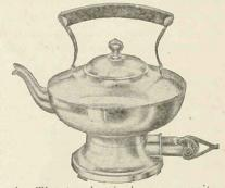
ized. The tea kettle has a capacity of two and one-half pints. It is made of drawn copper, spun into shape. The spout is of white metal. It has a bail handle, the sides of which are of steel and the grip is made of ebonized wood, shaped for convenient pouring. The kettle is finished outside in highly polished nickel in order to reduce heat radiation to a minimum, thus affording maximum heat production. The water may be heated wherever there is a lamp socket.
