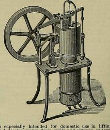
is especially intended for domestic use in lifting and forcing water from wells and cisterns, or from Croton pipes, to tanks on upper floor of buildings in city or country.
